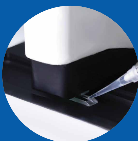
Load Cell Suspension into Sample Chamber
