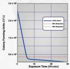
Adjustable pipettes were inoculated with S, aureus and placed in the UV Pipette Carousel. Individual pipettes were removed during the Auto-Decon To cycle at various intervals and rinsed to collect any residual contamination. The rinses were then plated and the CFU counted to determine the effectiveness of a single decontamination cycle.
