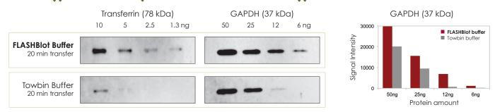
20 minute transfers of transferrin (high MW) and GAPDH (low MW) proteins were compared using FLASHBlot and Towbin buffers. Following Western blot analysis, the data show more efficient protein transfer with FLASHBlot Transfer Buffer.
