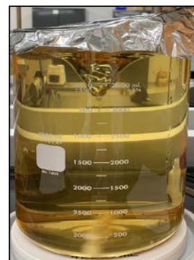
pH adjusted and make up the volume to 4 L (Before sterile filtration)
