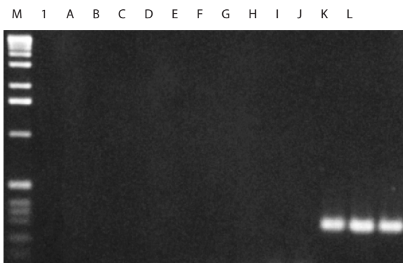
Figure 2. Amplification of a GC-rich template using the FailSafe™ PCR PreMix Selection Kit.
