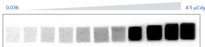
Figure 1. American Radiolabeled Chemicals Carbon-14 standard exposed to Storage Phosphor Screen for three hours then imaged on the Sapphire Biomolecular Imager.
