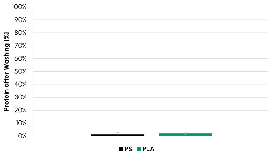
Figure 4: Amount of residual protein in the PS plates and 96-well microPLAte following a single washing step.
