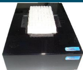
Racked cryogenically frozen tubes are scanned.
