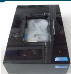
Without Cryoprotection™. Visible condensation.
