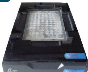
Without Cryoprotection™. Visible condensation.
