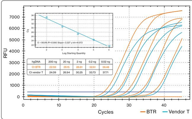
▲ **Accurate quantification over a wide linear range.** A qPCR assay was performed to evaluate the sensitivity, specificity and absence of non-specific amplification in non-template controls. Human genomic DNA was diluted (200 ng to 0.02 ng) and amplified using the CAPITAL qPCR Probe Mix and a mix from Vendor T.
