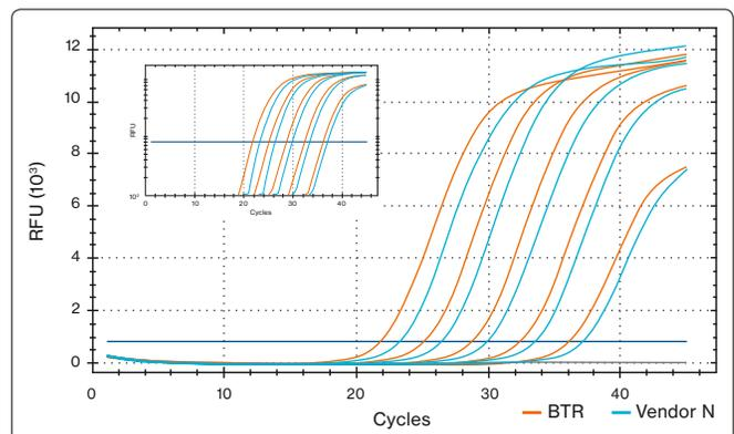
Sensitive and robust RT-qPCR. A one-step RT-qPCR assay was performed to evaluate low-input detection, specificity and absence of non-specific amplification in non-template control. RT-qPCR targets were quantitated with 10 ng to 1 pg total RNA targeting GAPDH. biotechrabbit CAPITAL qRT-PCR Probe mix showed earlier Ct in all dilutions compared to vendor N.
